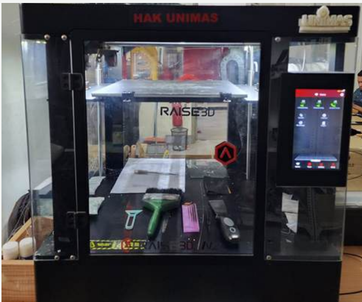
The Raise3D 3D printer in the faculty workshop – equipped with Dual Extruder and ready for innovative prints. Essential tools stored inside the printer chamber – including spatulas and brushes for post-print finishing.
